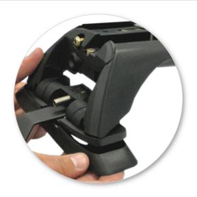
Fit rubber pads (supplied with fitting kit) to foot.
