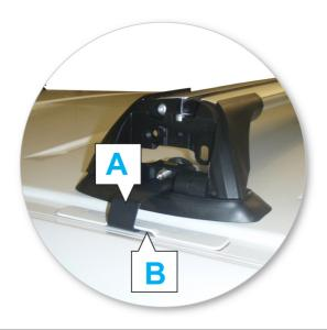
Clamp (A) hooks to the factory fitted fixed points (B) on roof of the vehicle.
