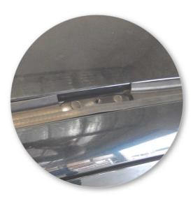
Re-install rubber ditch mould in roof channel. Remove all masking tape.
