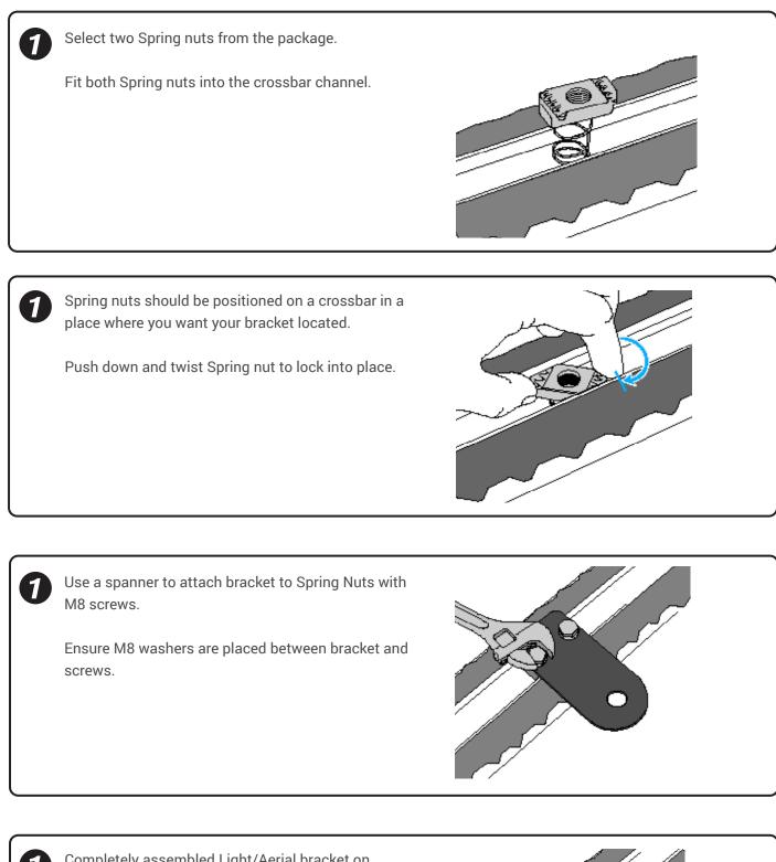
Completely assembled Light/Aerial bracket on crossbar.
