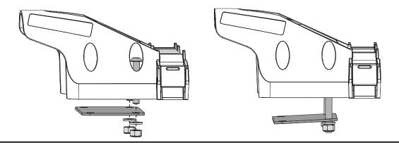
Position the Rod Holder Bodies on each crossbar with the strap/foam ends pointing towards each other. Slide the Clamp and Rod Holder assemblies onto crossbars as pictured. Install the remaining M6 x 40 mm Button Head Capscrews, M6 washers and M6 Nyloc Nuts into the outward facing holes. Tighten all Nuts to 4 Nm with a 10 mm spanner or a suitable Torque Wrench.
