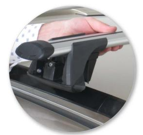
Place crossbar on vehicle. Minimum recommended spacing between the bars is 700mm (27 1/2") (unless otherwise stated).
