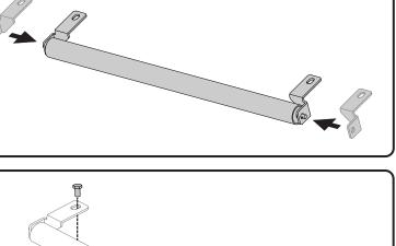
Attach using T-Nuts and Set Screws. Tighten Set Screws, ensuring there is a clearance between the roller and the bracket.
