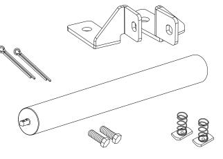
Fit left and right hand brackets onto roller shaft and position on roof bar
