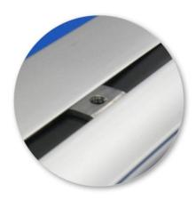
T-Slot nuts should be positioned on a crossbar in a place where you want your bracket located.
