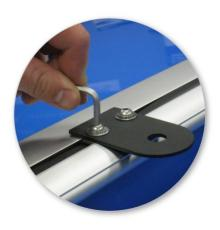
Use 4mm Allen key to attach bracket to T-Slot nuts with M6 screws.
